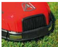
Paraurti e sensore ostacolo Bumper and obstacle sensor
