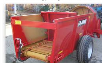
Sponda posteriore mobile ad avanzamento automatico Rear door advancing pushing manure to the turbine
