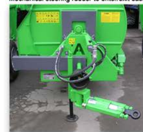
Timone sterzante meccanico Mechanical steering rudder to enter/exit easier in the row
